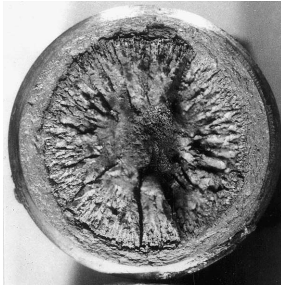
Fig. 5. Circumferential crack propagation patterns for a shaft under various applied torques.
